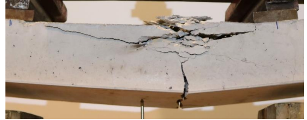
Fig. 20 – Failure mode of slab Ref Fire .
